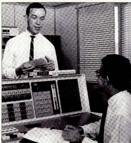
This photograph shows one of the computer operators, E Swoboda, seated at the operating console of the IBM 7090. The computer is controlled from here and monitor lamps indicate that it is functioning correctly. Looking over the console is H Klein, the senior operator.
