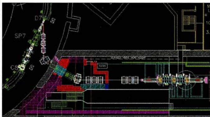
Layout of the planned Muon Ionization Cooling Experiment (MICE) at RAL, with the ISIS ring and pion-producing target at left. A muon beam produced from the decay of the pions is transferred to the MICE experiment on the right.
